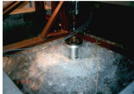
Fig. 6 – Air-water mixing and air entrainment in action
